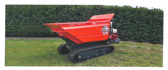
Engine: Honda GX390Power: 13 hp (10.4kw)
